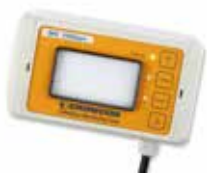
Crowcon F-Gas Detector Refrigerant Gas and SF 6 Detector
